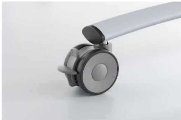
Swivel castor with kick pedal brake \varnothing 75 mm. Polypropylene support with thermoplastic rubber tread. Suitable for carpet floors. Load capacity (static) 120 kg.
